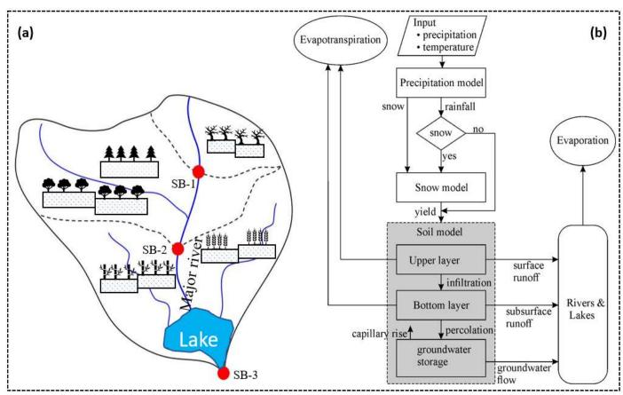
(a) Schematics demonstrating the watershed delineation for the WSFS model, its subbasins (SB-1, SB-2, SB-3), and the grid-cell discretization by soil type, vegetation, and elevation, (b) a two-layer soil moisture model with the major hydrologic processes for each soil-land-use class. Suomen ympäristökeskus
